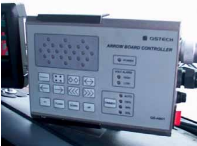
Real-time display on dashboard mounted controller
